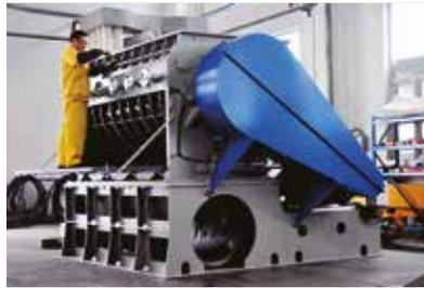
The granulators can be tailored to fit various applications, for example with oversized suction troughs in order to achieve a very high output.
