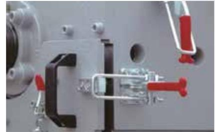
The ZERMA Quick Snap System allows the lower front plate section to be easily removed for granulator cleaning. The lower front plate section is held in position by two sturdy lever clamps.
