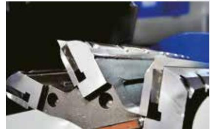
For abrasive applications the GSH granulators can be equipped with rotors with key parts manufactured from highly wear resistant steel as well as weld on hard facing.
