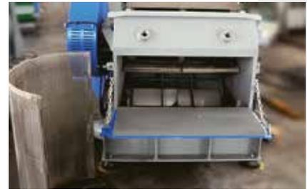
The base of the GSE 700 series makes the machine very sturdy, while maintaining the easy accessibility for maintenance and cleaning.
