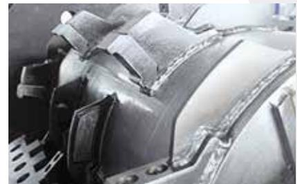
The combination of pre breakers and counter knives create a high impact power resulting in a high degree of disintegration and high throughput rates.
