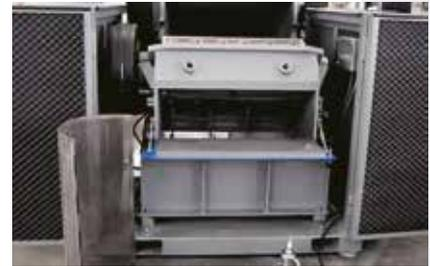
The user friendly design of the GSC series granulators allows quick and easy access to the cutting chamber for maintenance and cleaning.
