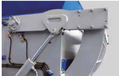
The ZSS series shredders benefit from sturdy ram construction incorporating heavy duty guide bearings and universal couplings for reliable operation.
