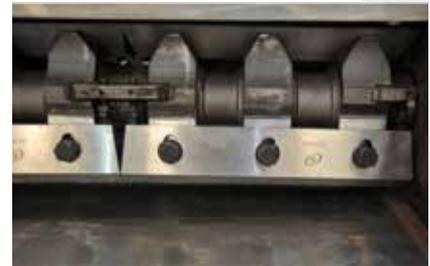
The granulator part uses a sturdy F+ rotor to ensure a good ingestion of the material flow while still being able to handle thicker and heavier particles.
