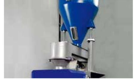
The material is fed into the Pulverizer by a vibrating dosing channel, the feeding rate is automatically adjusted based on the motors amperage and material temperature.
