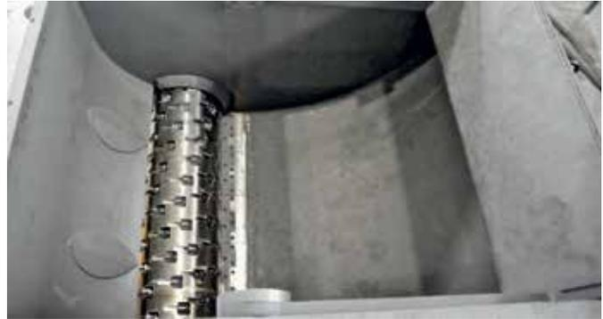
The internal ram design on the ZIS series allows the cutting chamber volume to be increased while keeping a small footprint. This makes the ZIS ideal for shredding big volume parts.
