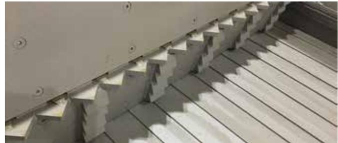
All ZERMA single shaft shredders are equipped with a serrated plate at the front of the hydraulic pusher. This helps ensure constant feeding of the material into the rotor with a variety of materials.
