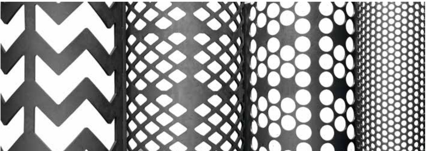
The shredders can be equipped with a variety of screen designs to tailor the machine to different materials. Common designs include round holes, square, diamond and zig-zag.
