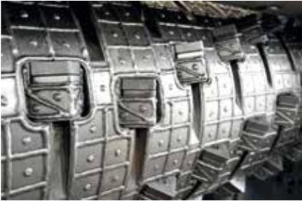
For heavy wear applications or abrasive materials weld on hard facing can be applied to the rotors and knife holders. Specially designed Tungsten Carbide blades can be used to extend the knife life when processing tires, MSW, or other contaminated materials.
