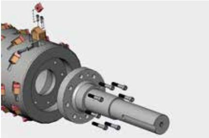
Rotor shafts and knife holders are bolted into the rotor to ensure easy reparability in case of accidents as well as acting as a safety braking point to prevent further damage to the machine.
