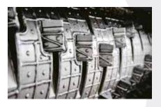
The ZTS and ZTTS shredders are equipped with a large diameter flat rotors with weld on hard facing. The knives are fixed in special knife holders fitted in machined pockets.
