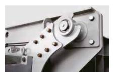
The oversized gearbox driving the rotor is supported by a very sturdy torque arm cushioning the shocks created while grinding.
